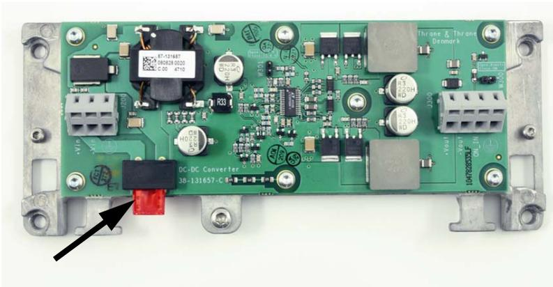
Figure 5: Replacing the fuse in the Power Converter
