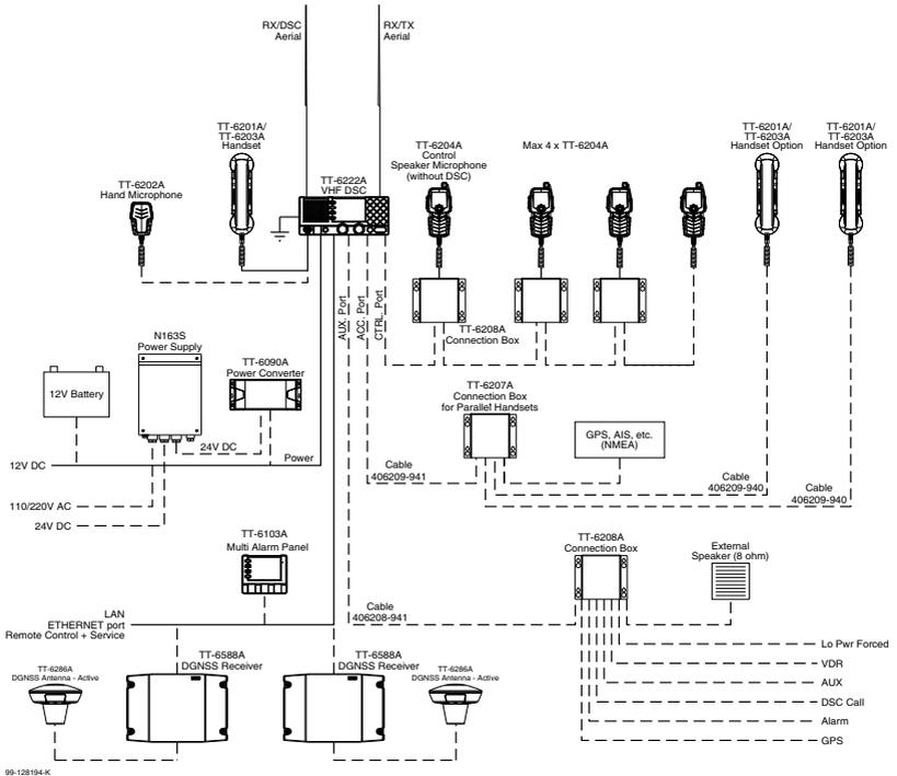
Figure 2: System configuration, example
