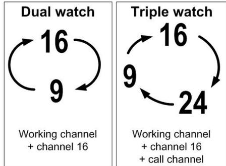
**To start the watch function** press the key **DW**. The radio enters the watch mode and the text WATCH with the channel numbers watched is shown below the current channel number.
