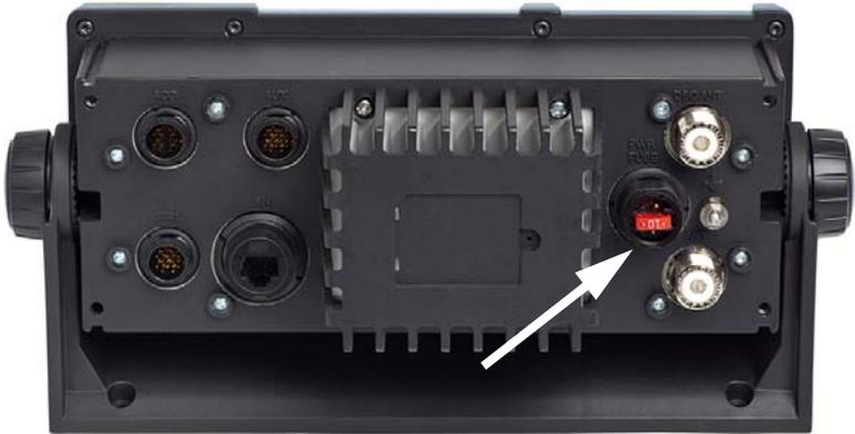
Figure 4: Replacing the fuse in the power connector
