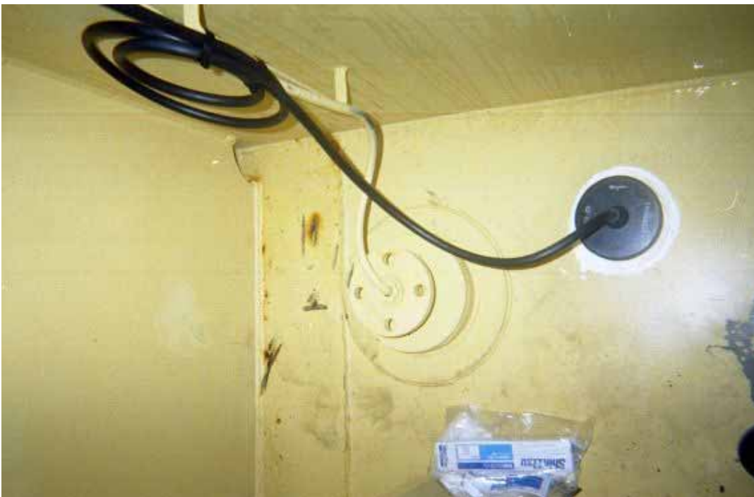
Photograph 4 Position where Transducer is installed inner Hull
