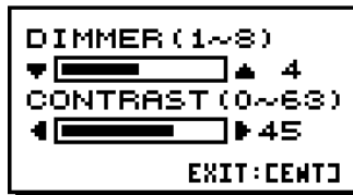
Figure 2-4 DIMMER and CONTRAST setting window
