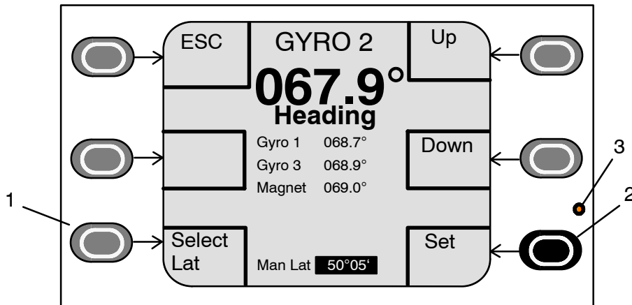
Figure 31: Controls and Indicators on the Operator Unit (after Man Lat has been selected)
