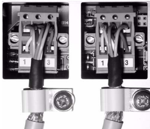
Figure 77: Example of a CAN1 bus - CAN2 bus connection (the Operator Unit is not the end device)
